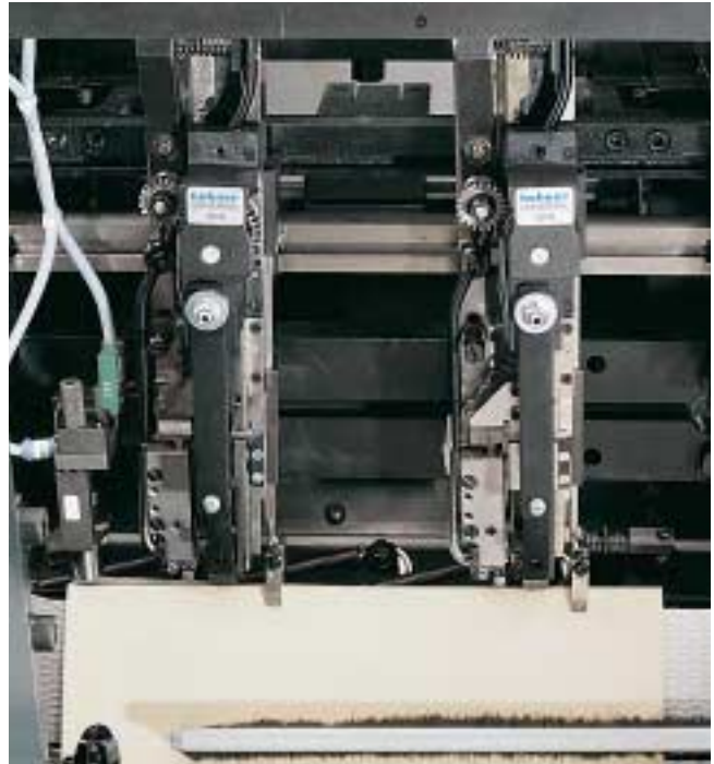
The stitching station is equipped with up to four stitching heads and comprehensive controls to create flexibility and safety.
