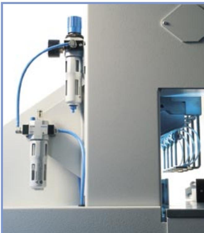
Professional drill bit lubrication with cooling system.
